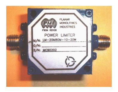
PLANAR MONOLITHICS INDUSTRIES, INC. has developed the PMI Model No: LM-20M80M-10-20W HIGH POWER LIMITER that operate from 25 to 80 MHz (other frequencies are available), with an input power level of 20 watts, Insertion loss of 0.5 dB maximum, VSWR of 1.5:1 typical and 1 Φsec recovery time packaged in a small package. The output limiting is +15 dBm maximum. The size is 1.0" x 1.0" x 0.40".
