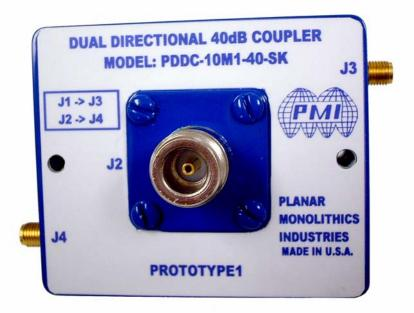
Planar Monolithics Industries, Inc. (PMI) is very proud to offer our latest product for your consideration. PMI Model: PDDC-10M1-40-SK is a 10 MHz to 1.0 GHz, 40dB, High Power, Dual Directional Coupler. The Directivity is 15dB Minimum at 1.0 GHz, Insertion Loss is 0.25dB Typical at 1.0GHz and the Return Loss is greater then 20dB across the band. The Coupling is very flat measuring -40dB at 10 MHz and -38.5 at 1.0 GHz. For more information, please visit PMI's website.
